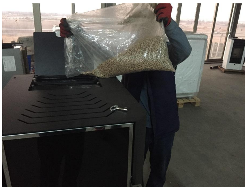
FUEL TANK LOADING
